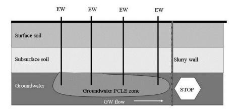
Figure 5. Example of Remedy Standard B groundwater response action where a control measure (slurry wall) is required to prevent the groundwater PCLE zone from expanding. EW is groundwater extraction well.
