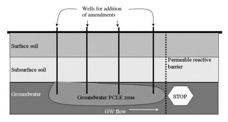
Figure 4. Example of Remedy Standard B groundwater response action based on decontamination (amendments, MNA and/or permeable reactive barrier)
