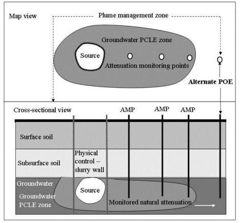
Figure 9. Example of Remedy Standard B plume management zone based on decontamination (monitored natural attenuation) and control (slurry wall). AMP is attenuation monitoring point.
