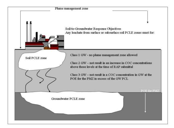
Figure 14. Soil-to-groundwater response objectives for circumstance when a PMZ has been approved for Class 2 or 3 groundwater
