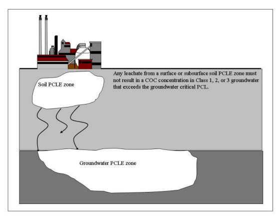
Figure13. Soil-to-groundwater response objective for circumstance when no PMZ has been approved.
